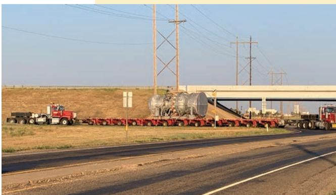
The case and rotor together weigh approximately 377,000 pounds. A heavy-haul trailer with 12 axles, 4 duals and 96 tires, shown here, was required to transport the unit from Abernathy, Texas, to Denver City, Texas. The new unit is a GE 7FA.03 gas turbine with DLN 2.6e combustion system. The unit is expected to provide years of reliable service for our Members.
